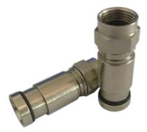
F Male Nickel Plated Brass 7/16 Hex 3/8-32 UNEF Threading 5 to 3000MHz 75 Ohm Nominal 90 V (at 60 Hz Continuous AC) -40 to +60 °C (-40 to +140 °F) FX-CT5087
